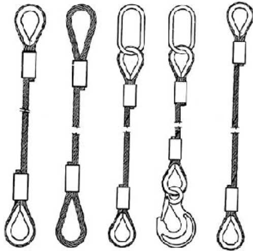
Various Configurations of Single Leg Wire Rope Slings
